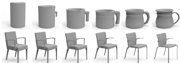
Fig. 17. Shape interpolation of cups and chairs with different topologies using our method. The first and last columns are the input shapes for interpolation.
